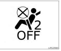
10. If the child restraint is installed on the front passenger seat, push the power switch to the ON position. The front passenger air bag status light should illuminate. If this light does not illuminate, see "Front passenger air bag and status light" (P.1-55). Move the child restraint to another seating position. Have the system checked. It is recommended that you visit a NISSAN certified LEAF dealer for this service.
